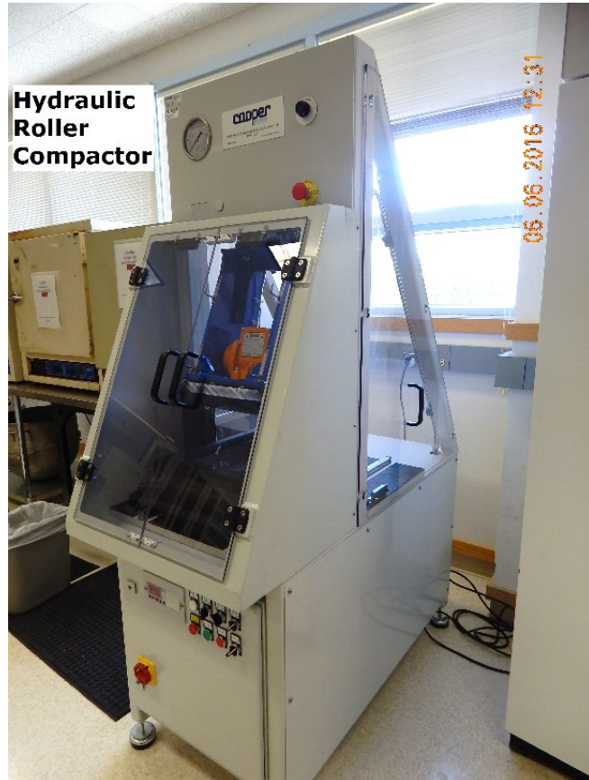
Hydraulic roller compactor simulating field construction
