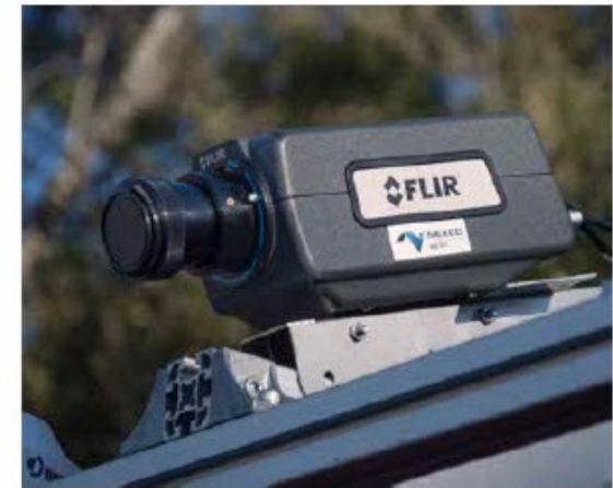
FLIR A6701sc camera used to create infrared delamination maps
