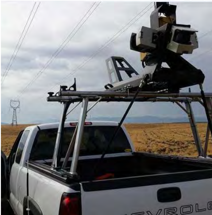
Mobile Lidar (Courtesy of Erlandson)
