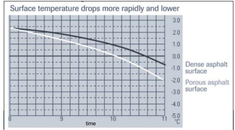
The insulating effect of PPPs inhibits heat transfer from the subgrade and can result in a frozen surface, while an adjacent DGP remains above freezing.
