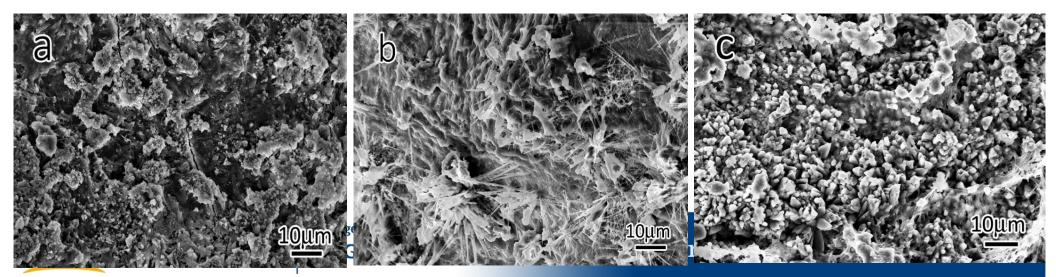
High magnification fracture surface SEM morphologies of the samples cored from SR431 site, a) moderate, and b) severe.
