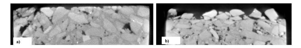
Mechanical keying a) CT image of DGP, b) CT image of DGP with chip seal.
