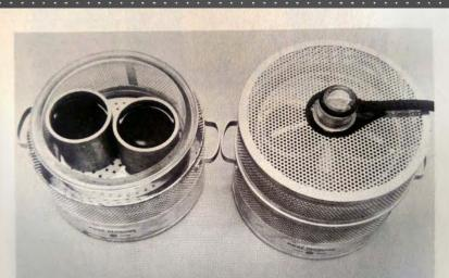
Fig. 7. Vacuum Soaking Apparatus
