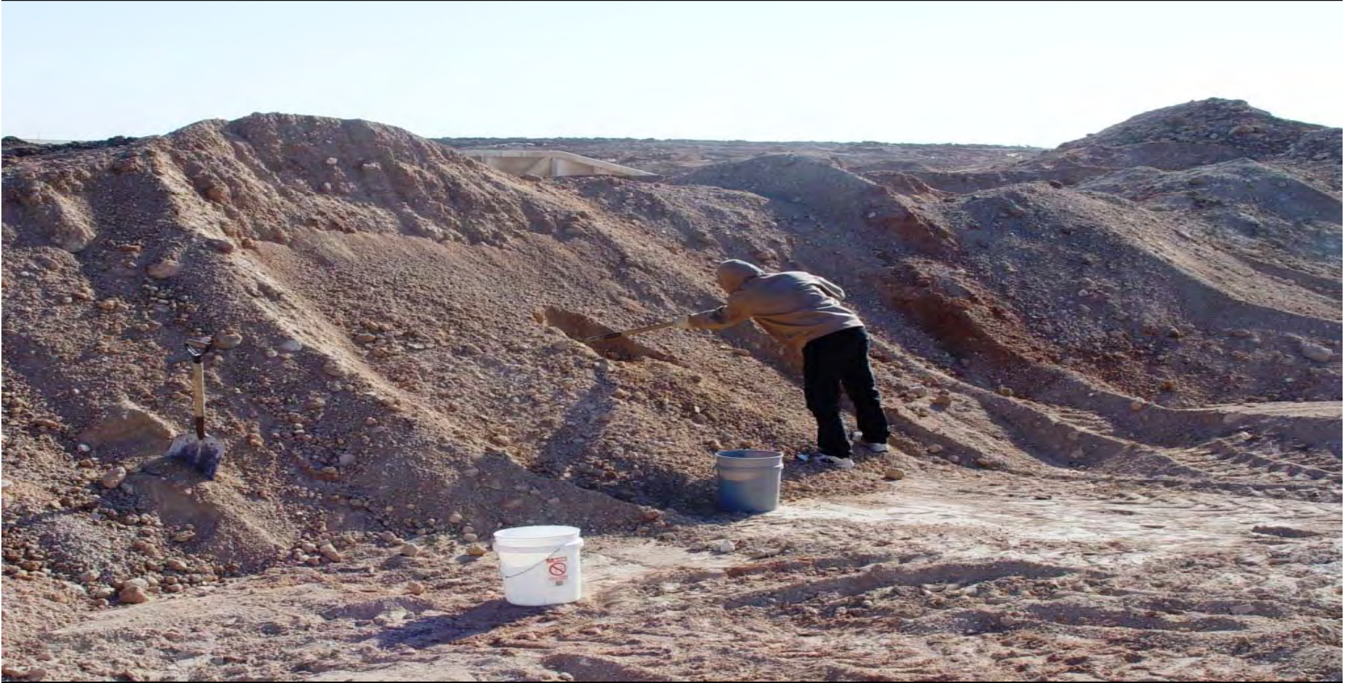
Sampling virgin aggregate stockpile at the Atlas Pit
