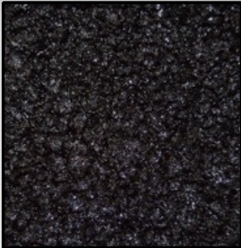
MICRO MIX sand mix provides better crack filling performance compared to cold mix; both filling and sealing; applicable to smaller cracks
