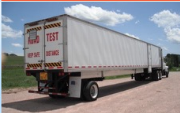
Rolling Wheel Deflectometer
