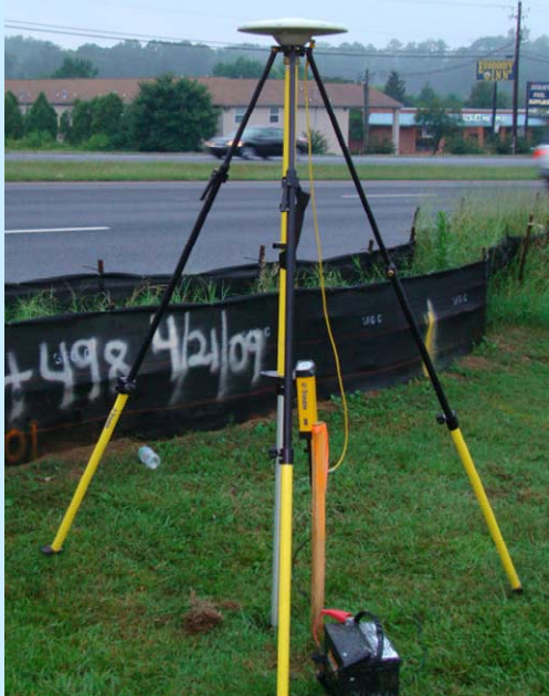
GPS Base Station
