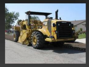
Improves existing materials in-place to provide greater structural support and reduction of imported material.
